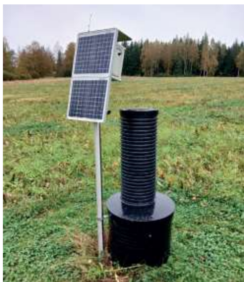
Figure 4. Remotely controlled and automated drainage control wells have been piloted in Finland, and several prototype systems have been developed. These systems can be powered by solar panels and operated without a direct connection to the electricity grid, with data transmission via mobile networks. Photo: Jari Kolehmainen.
